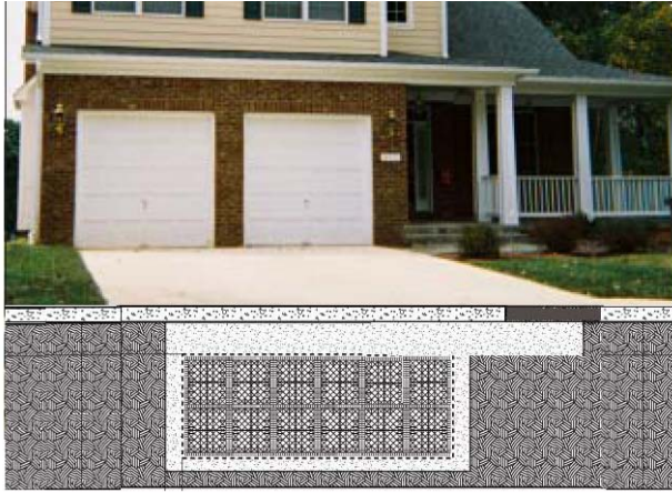
Figure 3. Infiltration chamber located below driveway (image provided by Atlantis Water Management Systems)
